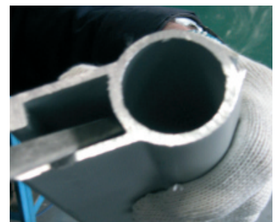
- Remove sharp edges -
