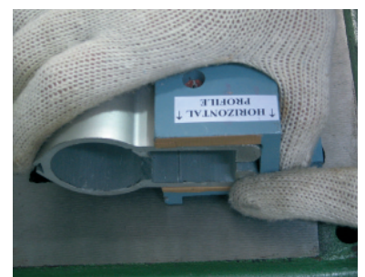
- Position in the boring template -
