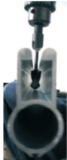
- Internal hole drilling -
